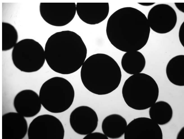
Figure 1 Photographs of the composite bead appearance.
